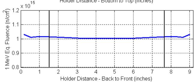
**Left Side:** Graphs depict the calculated 1 MeV equivalent neutron fluence profiles along centerlines of the FNI in the XY model
