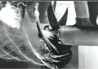
In this Navy water-tunnel experiment, the blades of a propeller produce cavitation bubbles.
